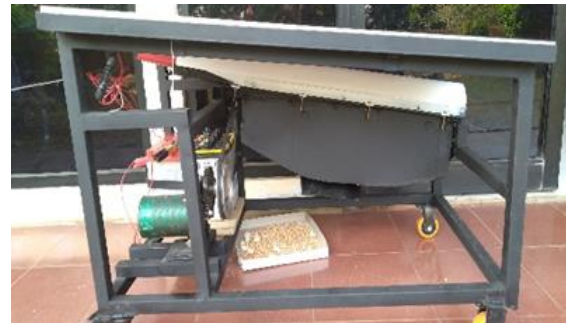
Figure 5. Previous Corn Sheller Machine Before Development
